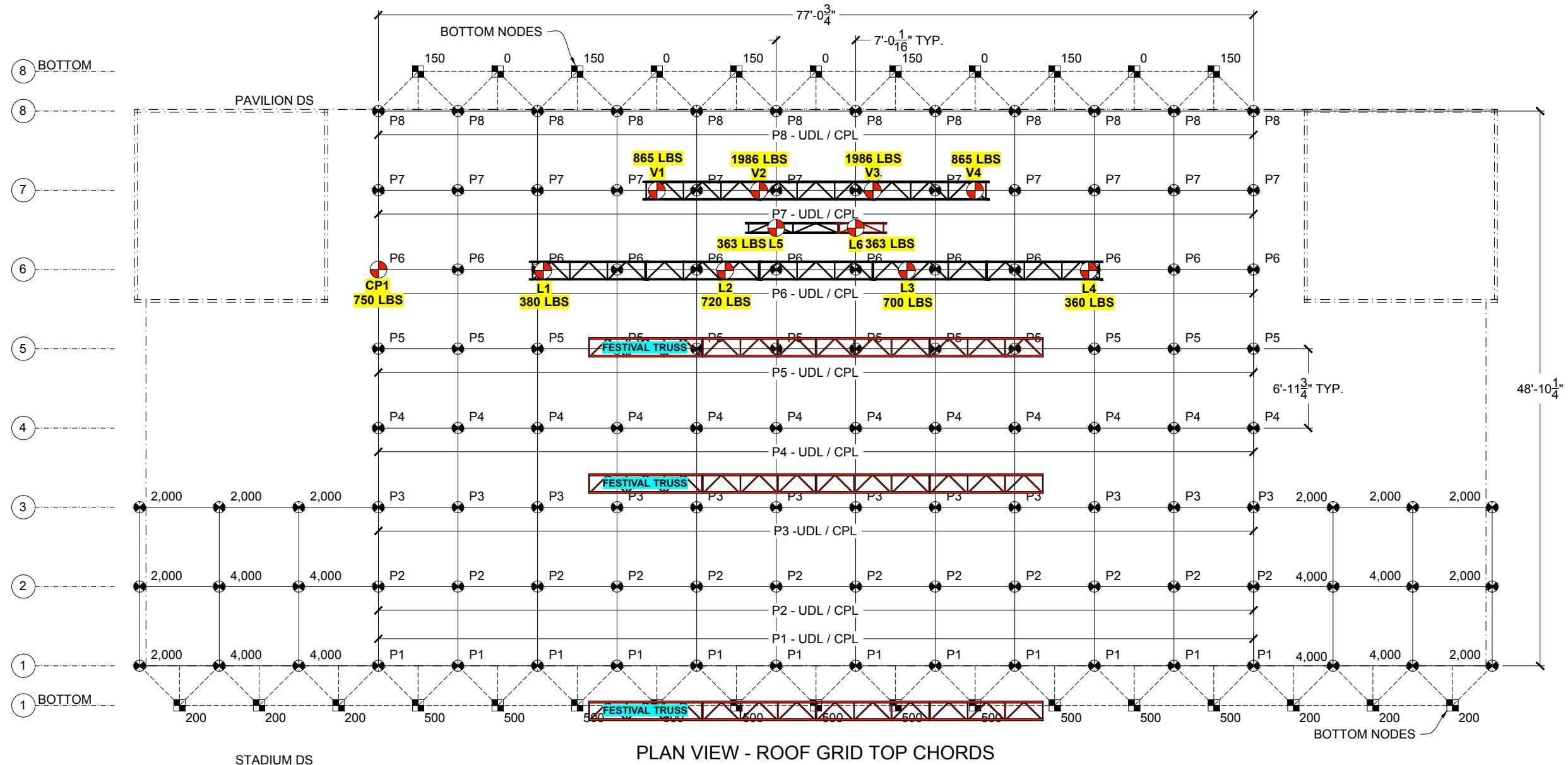
— FOR UDL EACH NODE DOES NOT HAVE TO BE LOADED
